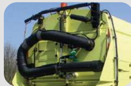
Manual suction system at the rear
