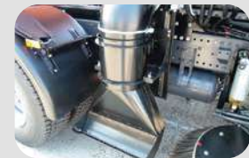
Blower nozzles can be directed manually or from cab
