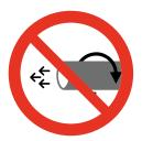
Pipes should never be dragged or rolled along the ground
