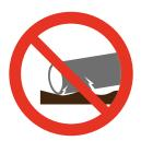
Pipes should never be dropped on to hard or uneven surfaces
