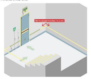
d) Directional indicators (arrows or the like) are to be mounted at changes in direction and at locations intended to lead persons out of, or from entering a dead end corridor
