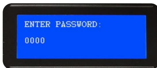
If password is entered correctly then system will enter to three main levels: SETTINGS AND PARAMETER, EVENTS and AUXILIARY INPUTS (user can shift between these three levels by UP/DOWN keys, then press ENTER to get into the selected one:
