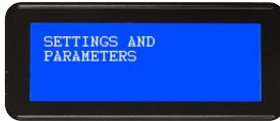
When user is in this level, he must press ENTER to go into the sub levels. The following sub levels will appear and user can shift between them by pressing up and down keys (default values can be seen between brackets [ ]), and user has to press ENTER again to go into the selected sub level to change the values and parameters. After changing parameters, user must press ENTER to save the new parameter, then press ESC to get out the sub level and go to another. These sub levels are:
