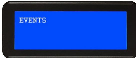
This level is to program the additional events only (main events/alarms are already programmed and can't be changed) see table 3. User can program three main actions for each event; audio signal, indicator (LED), and free contact. Some of these actions are not applicable with some events (see table 3). System has 10 programmable extra indicator (LED), and 8 programmable extra output relays. These events are:
