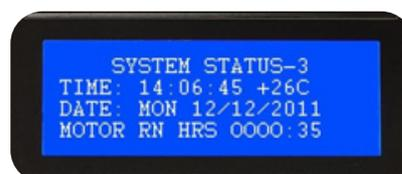
**Note:** For resetting motor running hours, user has to go to TIME / DATE RUNNING HOURS display, and then press ESC/REST key for 10 seconds.
