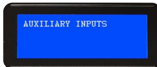
This level is to program additional  $n$  auxiliary inputs. User can program three main actions for each auxiliary alarm; audio signal, indicator (LED) and free contact. System has 10 programmable extra indicator (LED), and 8 programmable extra output relays.
