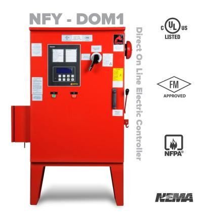
NAFFCO Electric Motor Controllers for fire pumps are listed by Underwriters Laboratories (UL file number EX15064), in accordance with UL 218 (Standard for Fire Pump Controllers), UL 508 (Standard for Industrial Control Equipment), NFPA 20 (Standard for the Installation of Stationary Pumps for Fire Protection), NFPA 70 (National Electrical Code) and relevant NEMA standards.
