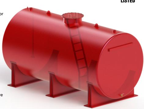
Applicable welding processes are Gas Metal Arc Welding (GMAW) and/or Shielded Metal Arc Welding (SMAW). Shell, Dish Head and Lift Lug material is carbon steel, ASTM A36 and legs shall be of carbon steel pipe, ASTM A53. Standard height for the tank leg is minimum 500 mm.
